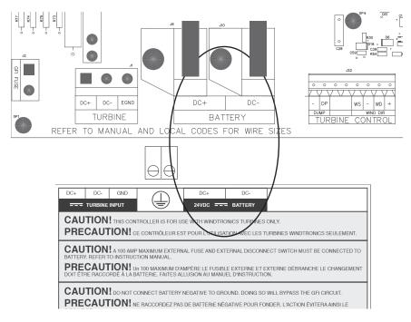
Figure 2.7 Battery Connection Location
